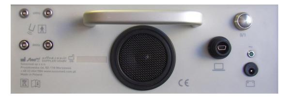
On the back of the device in the upper left corner are the transducers sockets marked respective of 4 and 8 MHz.
